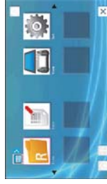
New teach pendant screen with a touch panel operable while wearing work gloves
