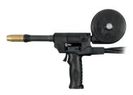
Spoolmatic® 15A Spool Gun #195 156 Spoolmatic® 30A Spool Gun #130 831 Ideal for aluminum welding jobs. Air-cooled 1-pound spool gun with 15-foot (4.6 m) or 30-foot (9.1 m) cable assembly. Rated at 200 amps at 100-percent duty cycle. For detailed information, see Spoolmatic literature, Index No. M/1.73.
